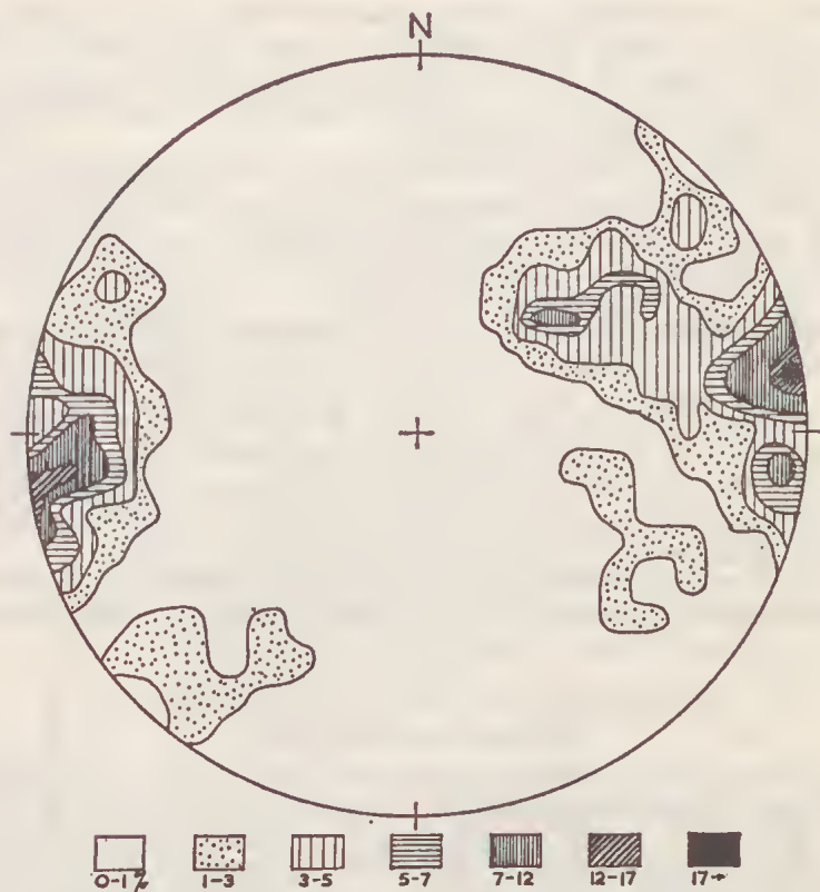
FIG. 6—Orientation of the long axes of 57 elongated pebbles from the Flowerdale Member.
